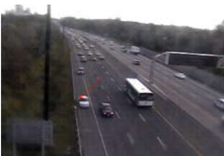
VisioPaD detects accidents on the highway and can identify stopped vehicles within 20 seconds
