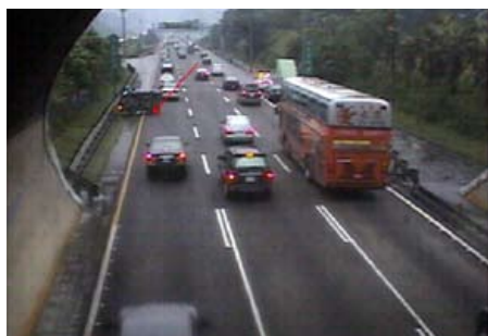
VisioPaD detects accidents on the highway and can identify stopped vehicles within 20 seconds
